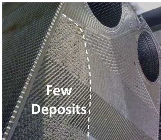
Fig. 8. Deposits formed on the surface of NT-plate.
