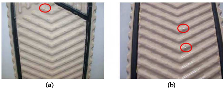
Fig. 14. Coated heat exchanger plates from heating section: (a) A2 coating, (b) A10 coating.
