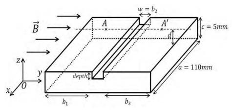
Fig. 7. Rectangular aluminium plate with a calibrated crack immersed in a uniform excitation field created by Helmholtz coils
