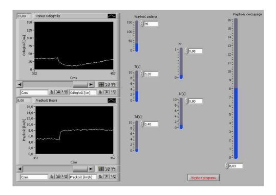
Fig. 4. LabView simulation of treadmill belt speed control
