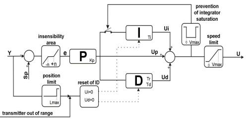
Fig. 3. PID controller algorithm
