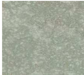
a. casting with no porosity
