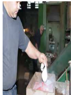
d. coating application by rag
