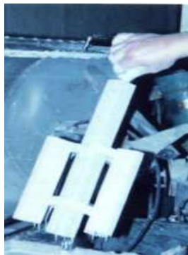
c. balancing the coating layer on the pattern
