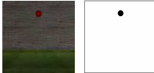
Fig. 4. A pair of images showing the ball in the simulated environment and the region where the object is detected by our tracking system satisfying the fuzzy color constraints.
