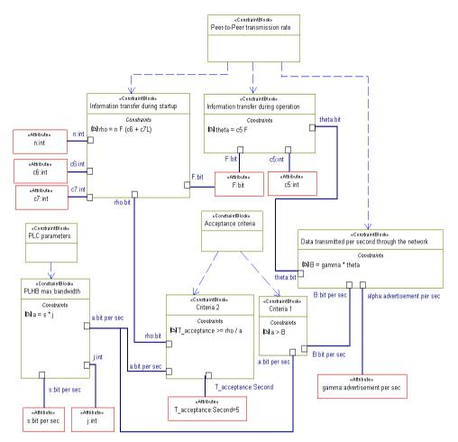
Fig. 12. Parametric diagram for system constraints
