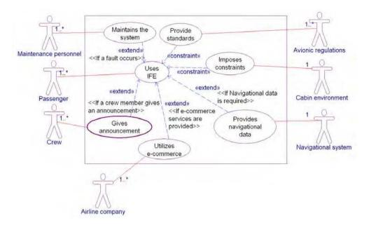
Fig. 8. IFE system Use Case diagram
