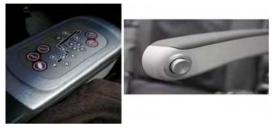
Fig. 3. Electronic Vs Mechanical seat adjustment
