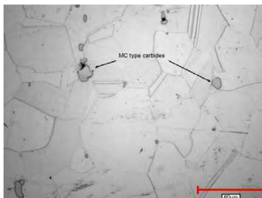
Fig. 12. Optical microstructure of as received 718 plus alloy (Vishwakarma et al, 2007).
