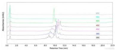
Fig. 8. Effect of temperature on mAb separation by CEX. The elution buffer (0.2 M sodium sulfate) was increased linearly on a ProPacWCX-10 column (4 x 250 mm).
