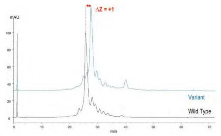
Fig. 4. Separation of mAbs differing by only one charge, a single amino acid change to primary structure. The elution buffer (0.5 M NaCl in 20 mM Tris, pH 7.3) was increased linearly on a ProPac WCX-10 column (4 x 250 mm), which was held at 50 °C and had a flow rate of 1 mL min<sup>-1</sup>.
