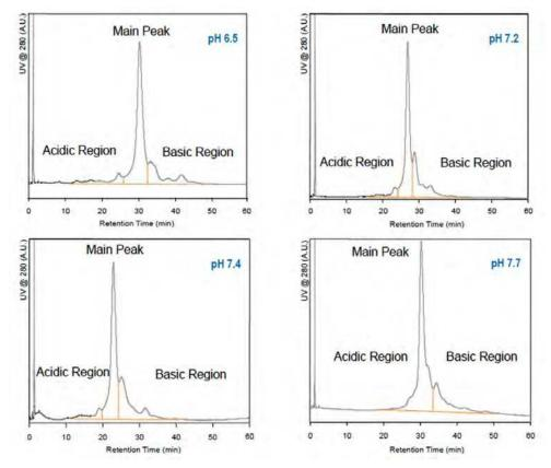
Fig. 7. Effect of mobile phase pH on mAb separation by WCX. The elution buffer (0.5 M NaCl) was increased linearly at 1 mM min<sup>-1</sup> at a flow rate of 1 mL min<sup>-1</sup> on a ProPac WCX-10 column (4 x 250 mm), which was held at 30 °C. Different initial salt concentrations were optimized for each pH value. Integration is shown, and main peak, acidic and basic regions are denoted.
