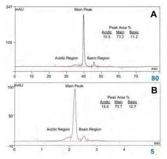
Fig. 10. Separation of a mAb using (A) a WCX column, 10  $\mu$ m and (B) a SCX column, 3  $\mu$ m, by pH gradient IEC. Each mAb was analyzed using the same buffers and gradient volume.
