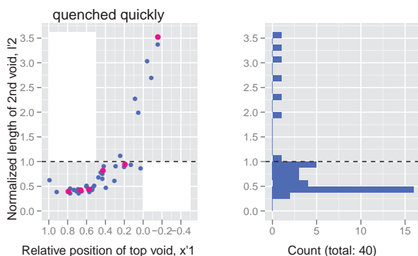
Fig. 16. Correlation between x'_1 and l'_2 (left) and histogram of l'_2 (right) for the samples pumped with 9W 1.48 \mu\text{m} light in which the fiber fuse was extinguished in a coating-free segment (see text). The red points are the results for samples (1) – (6) shown in Fig. 15.
