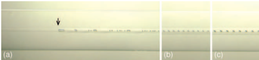
Fig. 6. Fiber fuse damage train in a standard single mode fiber (Corning SMF-28). After the ignition of the fiber fuse, the pump power of the laser ( 1.48 \mu\text{m} ) decreased from 7 W (c), 3.5 W (b) to \sim 1.2 W (a) until its self-extinction at the position shown by the arrow.
