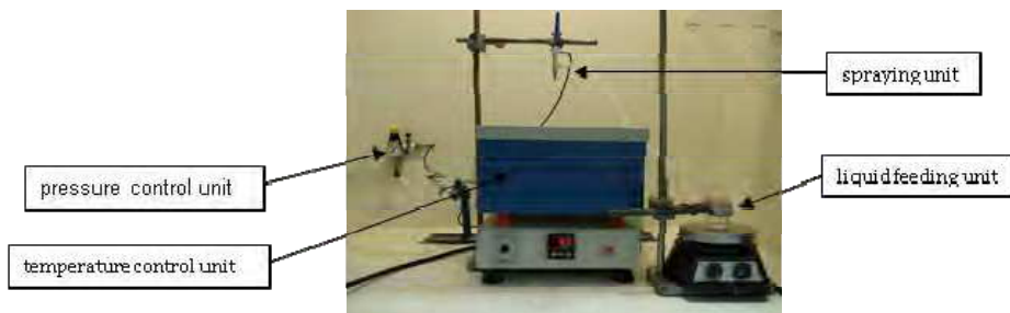
Fig. 3. Spray pyrolysis experimental apparatus.
