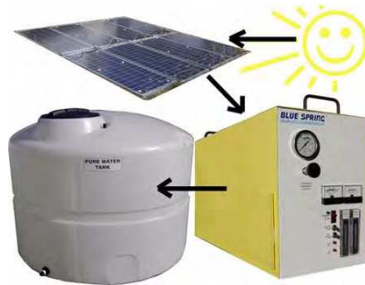
Fig. 7. Blue Spring Solar desalination system.
