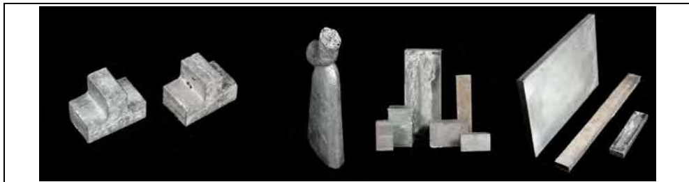
Fig. 14. 3D-parts of Al-alloy foams.
