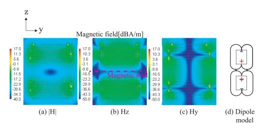
Fig. 4. Magnetic field distribution on a frequency of the even mode(12.3MHz) and equivalent dipole mode
