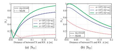
Fig. 17. Effect of transfer distance on the S parameters
