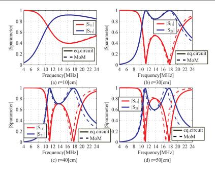
Fig. 19. Frequency characteristics of the S parameters( $\sigma = 10^8 [1/m \cdot \Omega]$ , h = r/16)
