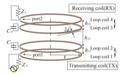
Fig. 11. Consideration model of indirect-fed type WPT structure
