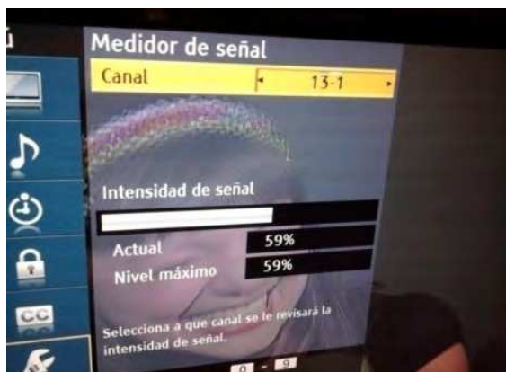
Fig. 14. Visualized images of HDTV reception antenna using the patch prototype, which is located on the house's roof.
