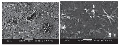
Fig. 6. SEM image of the surface of composite after immersion for 2h in 0.5 M H<sub>2</sub>SO<sub>4</sub> at 30°C in (A) absence and (B) presence of 400 ppm of DMABT. (Pinto et al. 2011)
