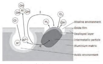
Fig. 2. Pitting corrosion mechanisms for the aluminium.
