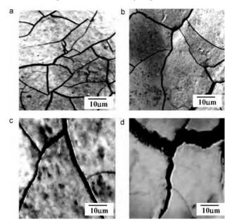
Fig. 4. Optical micrographs of the surfaces of 7075-T6 aluminium alloy specimens exposed to a deaerated 0.5 M NaCl solution at -685 mVSCE: (a) as-received specimen and (b), (c) and (d) specimens with grain sizes of 40, 130 and 290  $\mu$ m, respectively (El-Amoush, 2011)
