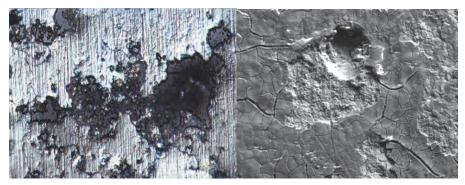
Fig. 3. SEM images showing the pitting corrosion for the aluminium
