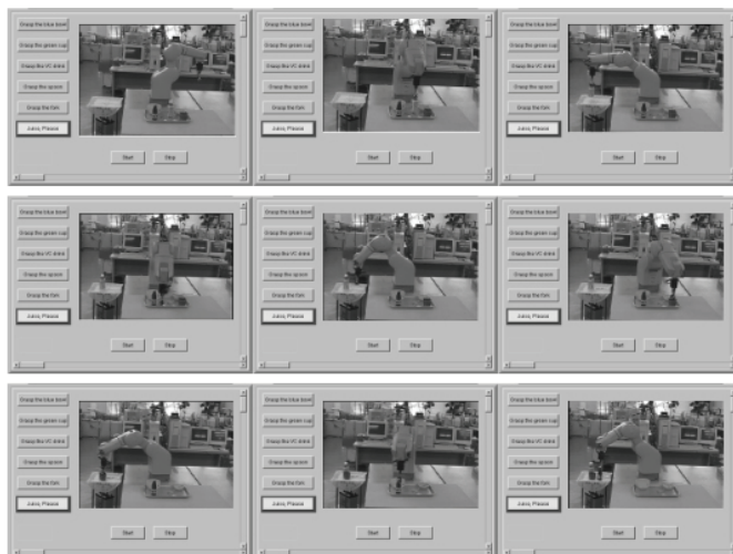
Fig. 10. Remote access to the hand-eye system; The remote user uses the telerobot system to manipulate the juice, fork, green cup and vitamin drink and put them to the tray mounted on the mobile platform.
