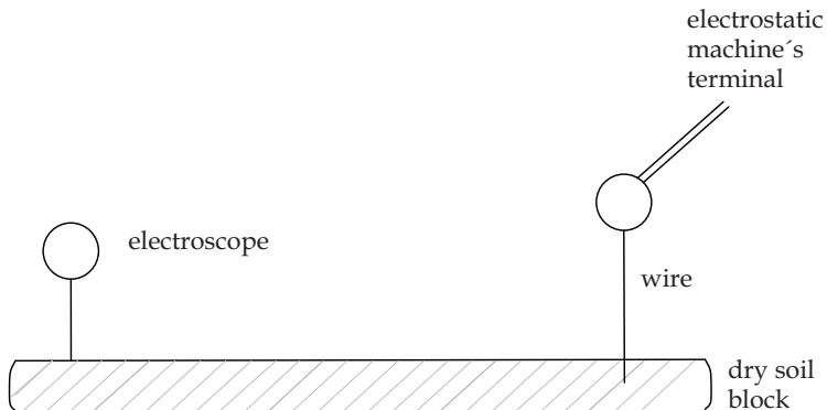
Fig. 14. A polarization charge is induced at the surface of a dry soil block
