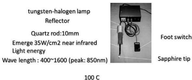
Fig. 20. KIRC-119: the plastic body has been replaced by a metal body to enable it to tolerate the long duration of the coagulation
