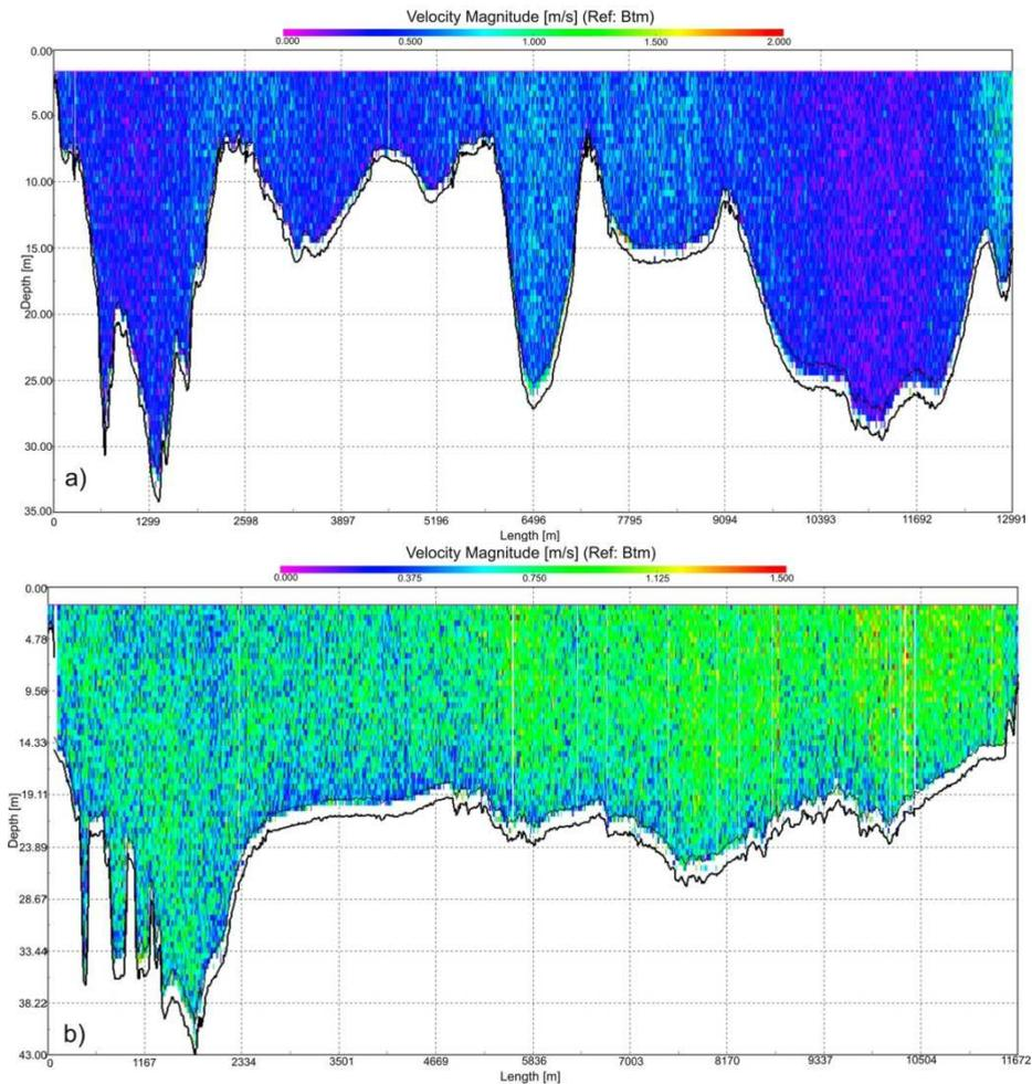
Fig. 2. Net discharge measured with ADCP (600Hz). a) North Channel profile, with  $Q = 1.3 \times 10^5 \text{ m}^3/\text{s}$  (12/05/2010), b) South Channel, with  $Q = 1.2 \times 10^5 \text{ m}^3/\text{s}$  (12/07/2010).
