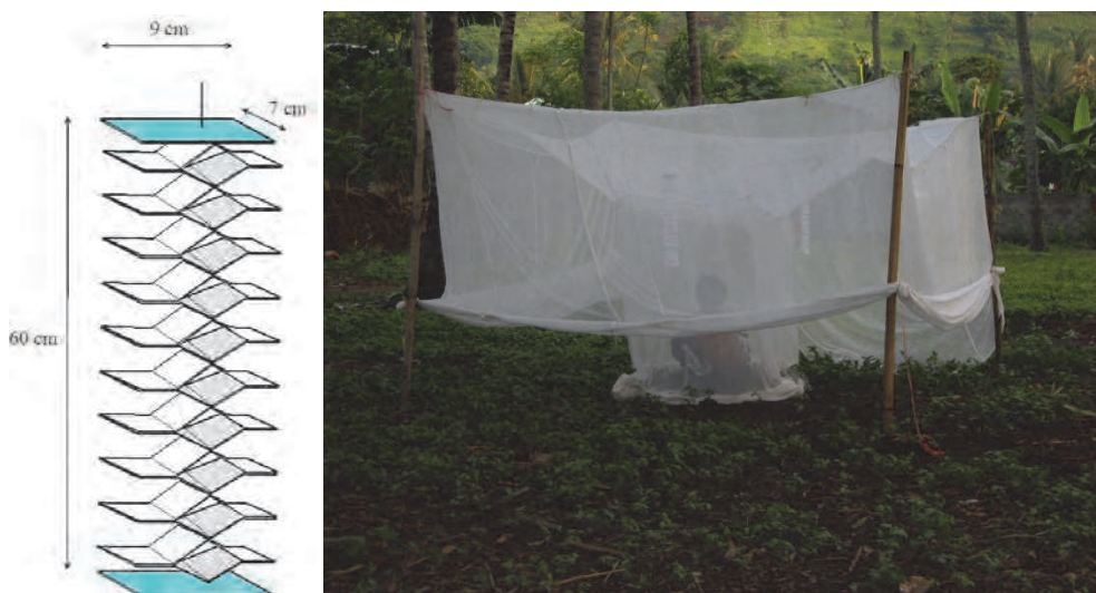
Fig. 1. Prototype Multilayer paper strip device impregnated with 200 mg of metofluthrin and outdoor human-baited collection with a double net (Strips were hung in a space between the inside and outside nets) (Kawada et al., 2004a).
