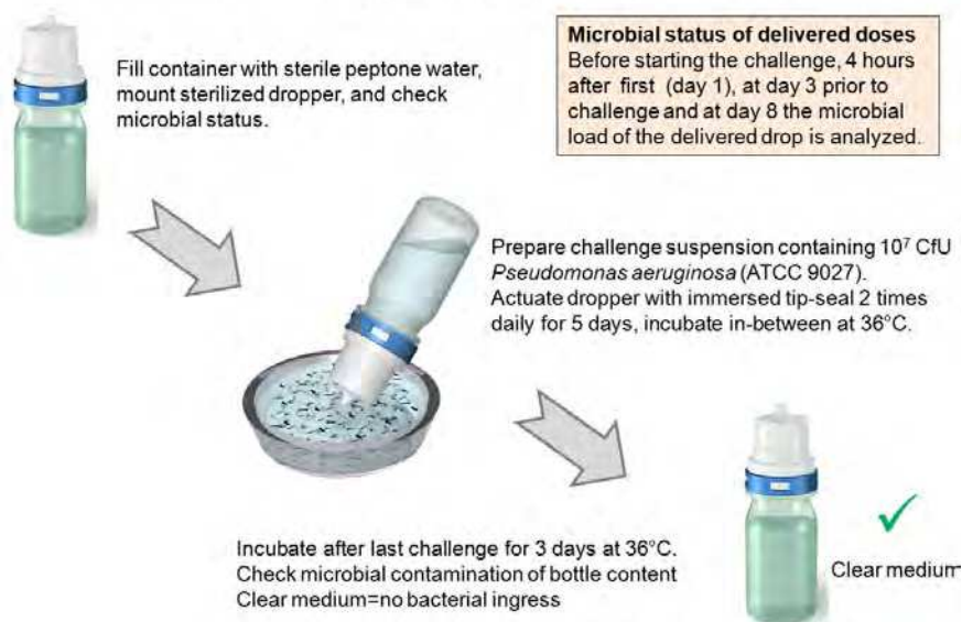
Picture 6. Microbial test to challenge the tip seal function and contamination of delivered doses with a preservative-free ophthalmic dropper.
