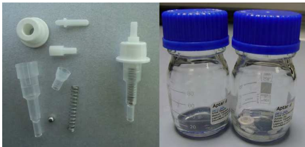
Picture 1. Parts for a standard pump and how it looks like when assembled. On the right side: soaking of parts in formulation to check compatibility. For demonstration just parts for one pump are depicted.
