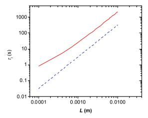
Fig. 4. The time required for the skin to reach values of the contact temperature of 0°C and 100°C without frostbitten or burning up respectively (see text), as a function of the hypothetical thickness of the gas layer evaporated at its surface. The solid and dotted curves correspond to the case of touching a cold (-196°C) and a hot (600°C) object, respectively Reproduced with permission from [Latin American Journal of Physics Education 2, 1, 15-17 (2008)].
