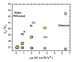
Fig. 3. Contact temperatures as a function of thermal effusivity calculated using Eq. (45) when touching with the hand at  $37\,^{\circ}\text{C}$  objects of different materials at  $0\,^{\circ}\text{C}$  (circles) and  $1000\,^{\circ}\text{C}$  (squares). Reproduced with permission from [Latin American Journal of Physics Education 2, 1, 15-17 (2008)]. Values of the thermal effusivities have been taken from [Salazar, 2003]
