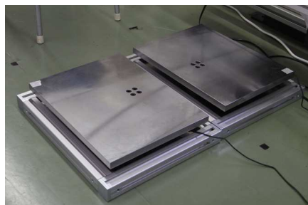
Fig. 5. Force detection plates for measuring feet pressure
