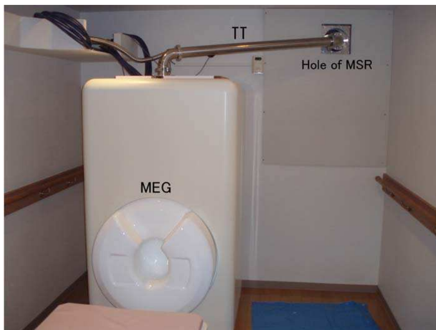
Fig. 13. Multi-pipe TT of the HCS installed on the commercialized MEG (PQ1160C, Yokokawa Electric Cor. Inc., Japan). As the TT has 1/2 inch insert tube, there was no need to modify the MEG to install the HCS. TT is twisted twice to use the ventilation hole located upper light to get through the MSR. It is tilted 5 degrees to get the LHe drop to the dewar.
