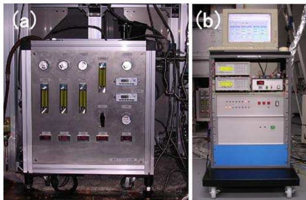
Fig. 12. Hardware of the gas control system of the HCS (a), and computer to control the gas flow together with temperature monitors and Liquid helium level meter (b).
