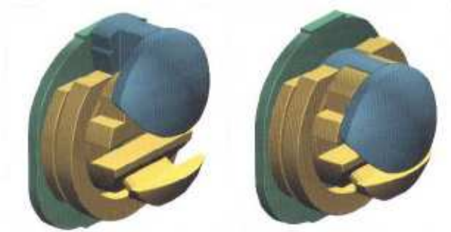
Fig. 6. Edgelok bracket in open and closed positions.
