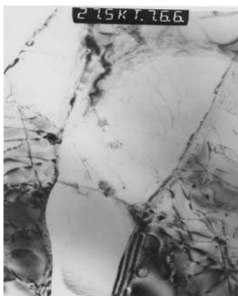
Fig. 8. TEM micrograph of Al 6013/SiC interface showing dislocation generations
