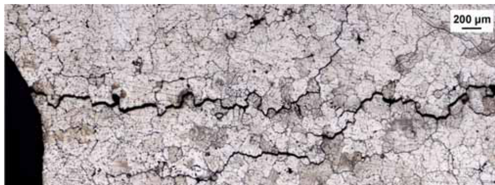
Fig. 14. Fracture path developed by coalescence of shrinkage porosity due to quenching of liquid phase
