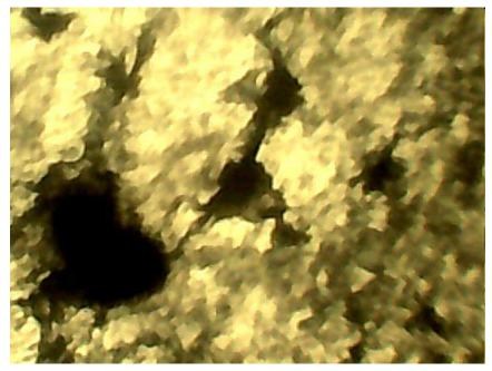
Fig. 6. Gas porosity in aluminium casting at 1000× magnification
