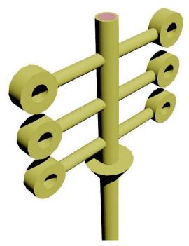
Fig. 9. An investment mould "tree", simplified structure is characteristic of the countergravity technique
