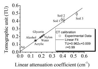
Fig. 1. Computed tomography (CT) calibration curve for <sup>241</sup>Am gamma-ray radiation. Error bars represent the standard deviation of the measurements. Soil 1, 2 and 3 are sand, clay loam and clay sieved soils.
