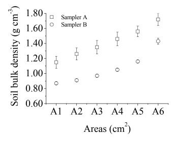
Fig. 11. Soil bulk density ( $\rho_s$ ) variation with the cylinder diameter for the schematic areas (A) presented in figure 9 for the quantitative image analysis. Error bars represent the standard deviation of the mean (n=5).
