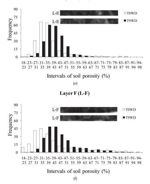
Fig. 13. (a-f) Changes in soil porosity ( $\phi$ ) along soil sample depth. T0WD and T9WD represents soil samples not submitted to wetting and drying (W-D) cycles and submitted to 9 W-D, respectively. Values of  $\phi$  represent average of six replicates. The layer pictures (L slices) presented on the graphs is only illustrative for the specific sample presented in figures 12a and 12c.
