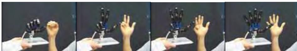
Fig. 12. The copycat hand can ape and imitate human hand motions at high speeds and with high accuracy.
