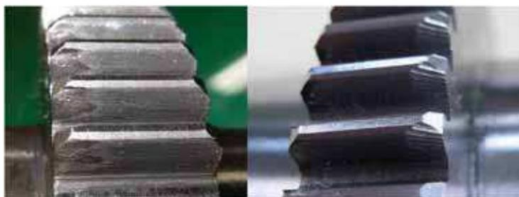
Fig. 8. Gear tooth worn by misalignment
