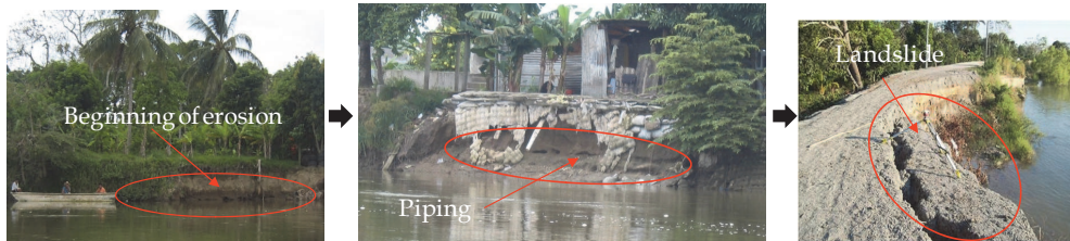
Fig. 3. Evidences of instability in river banks caused by erosion (Auvinet & Lopez-Acosta, 2010)
