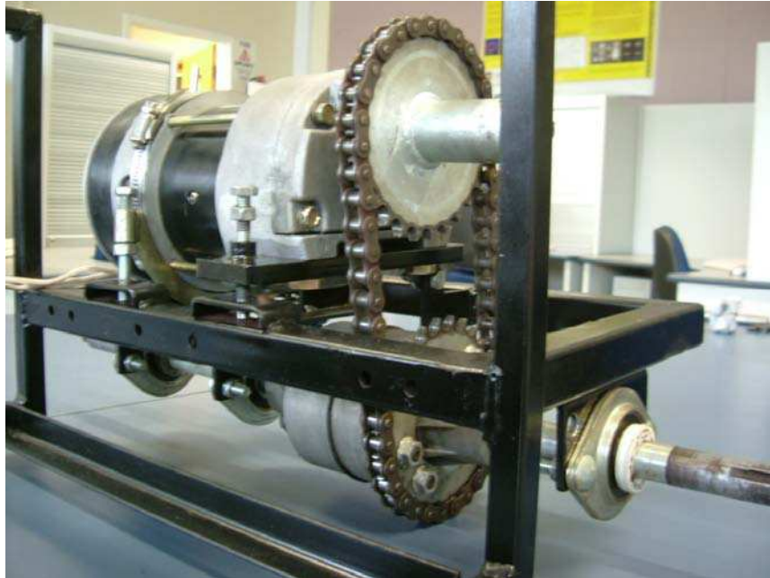
Figure 7. Mounted drive system showing chain tensioning method
