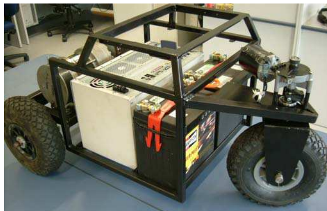
Figure 9. Complete chassis and drive components
