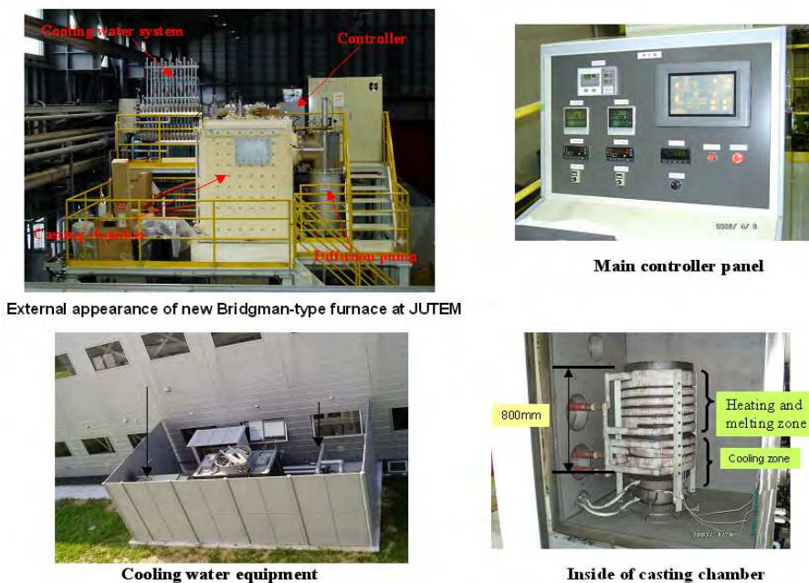
Fig. 22. New Bridgman-type furnace
