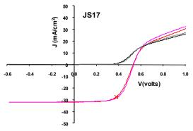
Fig. 13. J-V curves for the best Cu(In,Ga)Se<sub>2</sub> thin film device prepared with a CdS bath solution based on CdCl<sub>2</sub>
