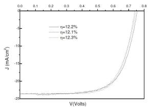
Fig. 16. J –V characteristics of three CdS/CdTe solar cells made with CdS layers grown with  $R_{tc}$  = 5 during the CBD-CdS growth process
