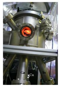
Fig. 8. Thermal co-evaporation system with Knudsen effusion cells to deposit  $Cu(In,Ga)Se_2$  thin films
