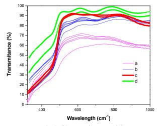
Fig. 4. Transmission response of CdS films as a function of the position inside the reactor
