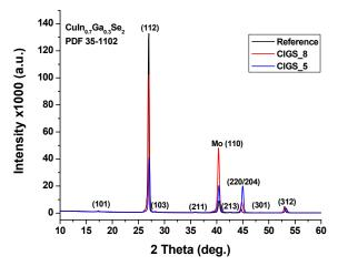
Fig. 10. XRD pattern for Cu(In,Ga)Se<sub>2</sub> thin films thermal co-evaporated
