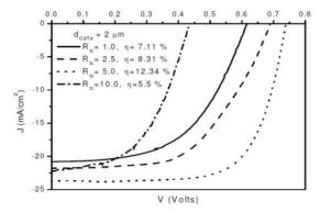
Fig. 17. Typical J –V characteristics of CdS/CdTe solar cells under illumination at 100 mW cm<sup>-2</sup>, with  $R_{tc}$  as a parameter
