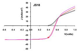
Fig. 14. J-V curves for the best  $Cu(In,Ga)Se_2$  thin film device prepared with a CdS bath solution based on CdSO<sub>4</sub>
