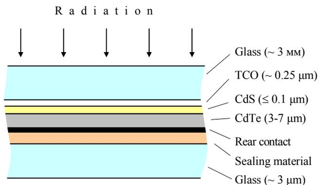
Fig. 12. Cross-section of thin film solar cell CdS/CdTe.
