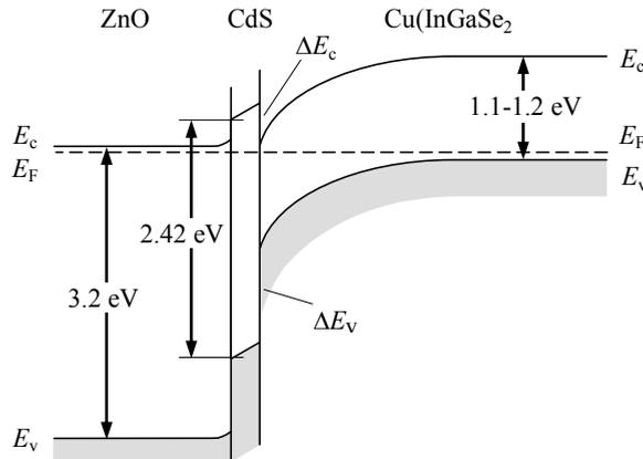
Fig. 10. Energy diagram of ZnO/CdS/CuIn<sub>x</sub>Ga<sub>1-x</sub>Se<sub>2</sub> solar cell.
