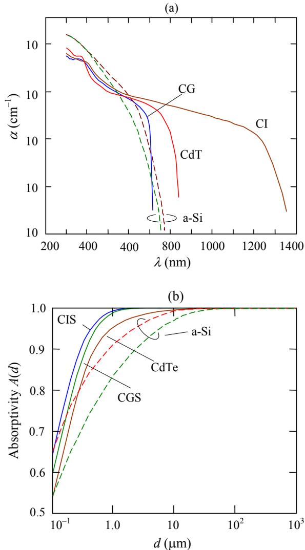
Fig. 4. Absorption curves (a) and dependence of absorptivity of AM1.5 solar radiation in the  $h\nu \geq E_g$  spectral range on the absorber layer thickness  $d$  (b) for amorphous silicon (a-Si), cadmium telluride (CdTe), copper-indium diselenide (CIS) and copper gallium diselenide (CGS) (Han et al., 2007; Paulson et al., 2003; Gray et al., 1990; <http://refractiveindex.info/a-Si>).
