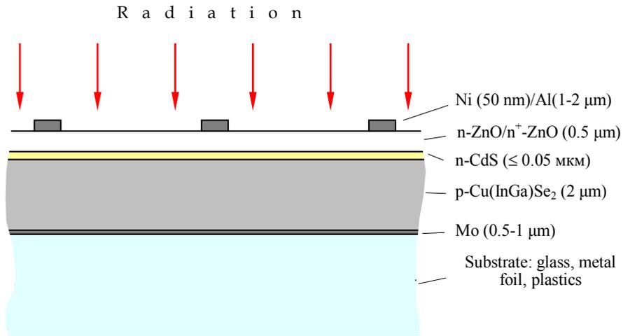
Fig. 9. Schematic cross section of a typical Cu(In,Ga)Se<sub>2</sub> solar module.
