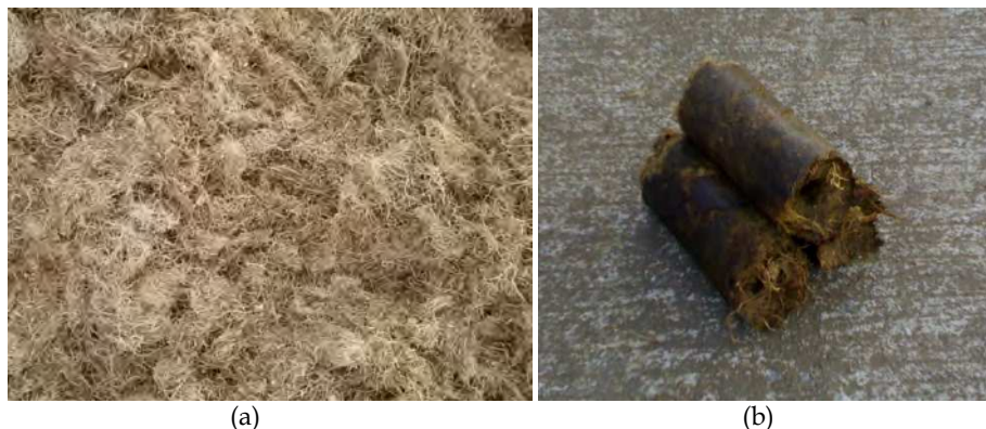
Fig. 9. PEFB before (a) and after (b) pelletizing
