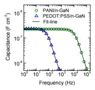
Fig. 6. C-f characteristics of TCP/epi.-GaN heterojunction solar cells.
