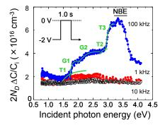
Fig. 7. DLOS spectra of PANI/epi.-GaN heterojunction solar cell.
