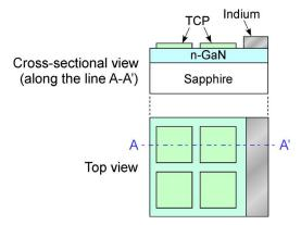
Fig. 2. Schematic of TCP/epi.-GaN sample.
