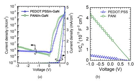
Fig. 4. (a) *J-V* characteristics and (b) Capacitance-voltage plots of TCP/GaN heterojunction solar cells.
