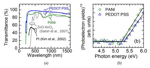
Fig. 3. (a) Optical transmittance spectra of PEDOT:PSS and PANI films. The transmittance spectra of ZnO-SnO<sub>2</sub> (Satoh et al., 2007) and semi-transparent Pt (Kim et al., 2002) thin films are also shown for comparison. (b) Photoelectron emission yield spectra of PEDOT:PSS and PANI films.
