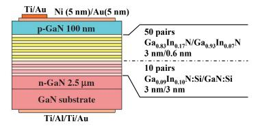
Fig. 1. Schematic of  $In_xGa_{1-x}$  N-based solar cell exhibiting 2.5% conversion efficiency (Kuwahara, 2011).
