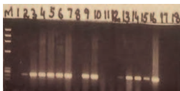
Fig. 7. Ethidium Bromide stained agarose gel showing PCR products of EBV-DNA amplified with primers specific for gp200 region.
