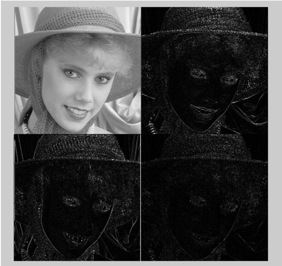
Fig. 12. Single level wavelet decomposition
