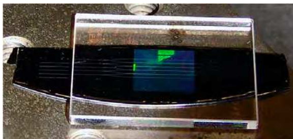
Fig. 24. Fabrication of Bragg gratings by UV exposure (KrF laser at 248 nm) through a phase mask. The major length of the diffractive area of the phase mask is 1 cm.
