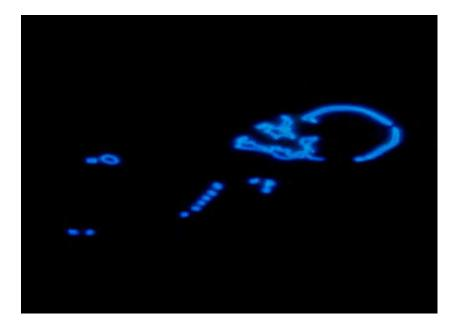
Fig. K. Slice showing the laser beam during the hardening process of the photo sensible resin on SLA VIPER Si
