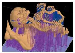
Fig. C. Virtual 3D model of skeleton including support structures for the Stereolitography process.
