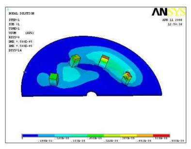
Fig. 10. Displacement analysis of the core
