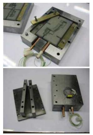
Fig. 14. Tool assembly components and the steel frames
