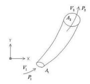
Fig. 4. Schematic representation of flow continuity
