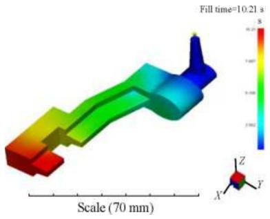
Fig. 18. Wax model filling time
