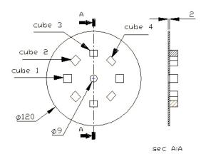
Fig. 5. Geometrical dimensions of the moulding
