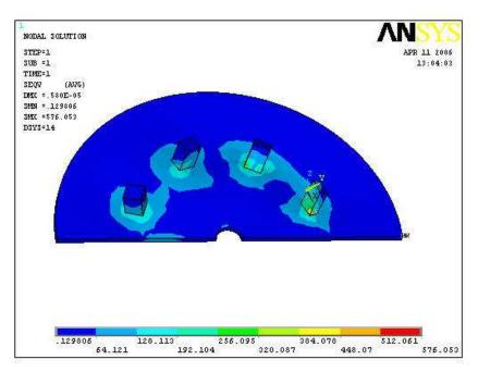
Fig. 11. Von-Mises stress analysis of the core
