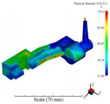
Fig. 20. Wax model freeze time
