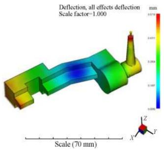
Fig. 26. Wax model warpage and shrinkage after ejection
