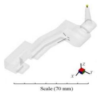
Fig. 17. Wax model weld lines
