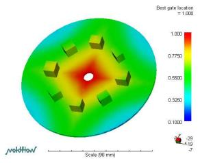
Fig. 6. MoldFlow analyses for sprue bush location
