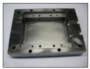
Fig. 22. Base plate machined into a rectangular pocket
