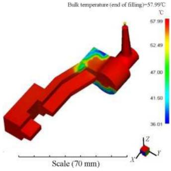
Fig. 19. Wax model temperature distribution
