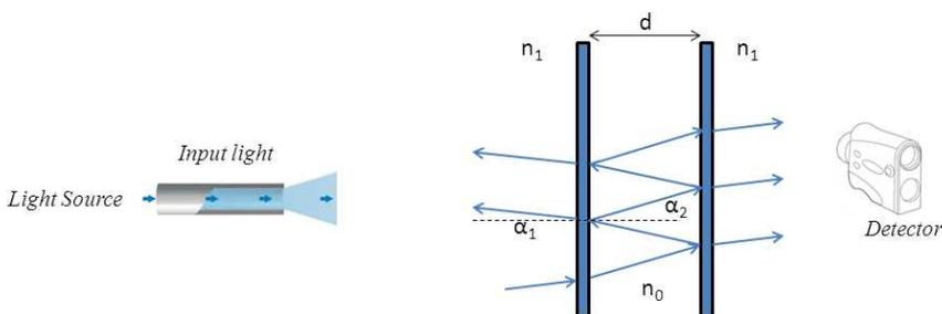
Fig. 1. Schematic representation of a Fabry-Perot interferometer.
