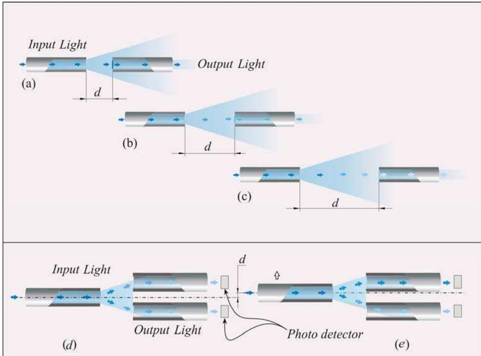
Fig. 4. Schematic representation of intensity-modulated FOSs realized with two fibers or more. The intensity of the coupled radiation of the two fibers is function of their distance  $d$ : if  $d$  increases the intensity of collected light decreases (a, b, and c). Sensors' performances can be improved using differential configuration (d, and e).
