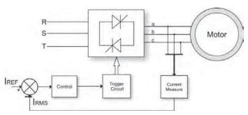
Fig. 5. Basic block diagram of the current control technique.
