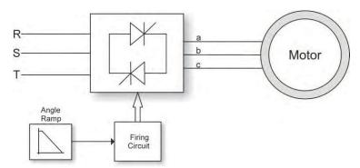
Fig. 3. Basic block diagram of the voltage-ramp technique.
