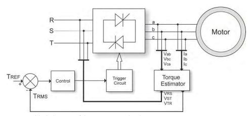
Fig. 7. Basic block diagram of the torque control technique.
