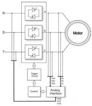
Fig. 2. Basic diagram of a soft-starter.
