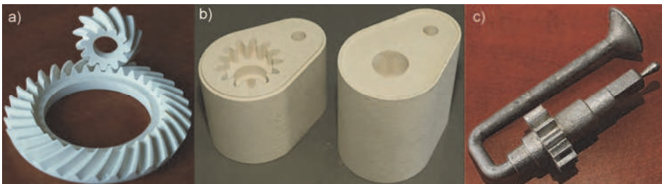
Fig. 6. Models produced by 3DP method: a) gear wheels, b) gear wheel casting mould, c) cast made in the mould from Al alloy
