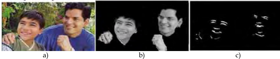
Figure 2. Results of Skin color segmentation a) Original Image b) Potential face regions in gray scale image c) Sobel Filtered Binary image
