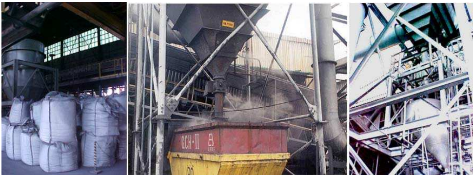
Fig. 15. Petro coke handling problem at Albras, in left bake furnace, in center and in the right bag house dust discharge at the rodding shop - source: Albras Alumínio Brasileiro SA.
