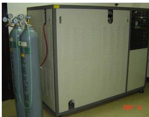
Fig. 11. Three-path-equipment of alkali metal charging (figure 10)
