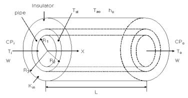
Fig. 1. Insulated pipe
