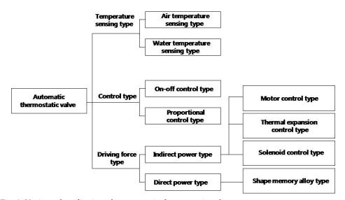
Fig. 8. Various classifications for automatic thermostatic valves
